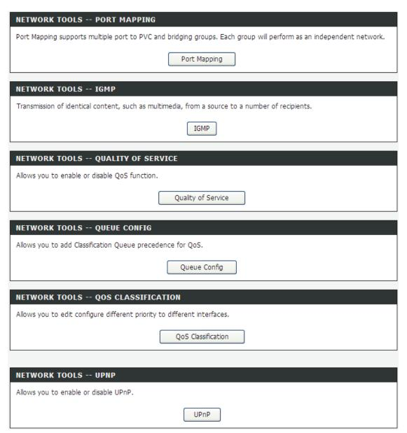
In the **NETWORK TOOLS** page, you can configure port mapping, IGMP, quality of service, queue, QoS classification, UPnP, ADSL settings, SNMP, TR-069, and certificates through clicking the navigation.
