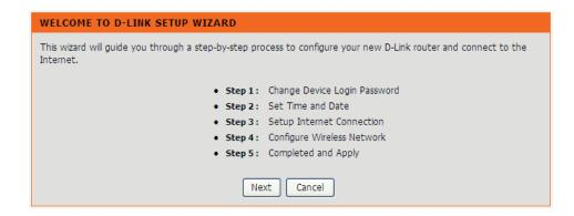
There are four steps to configure the device. Click **Next** to continue. Change the password for logging in to the device. The default password is **admin**. To secure your network, modify the password
