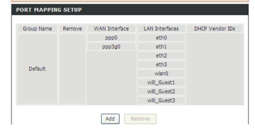
Click **Add** to add port mapping. The page shown in the following figure appears. The procedure for creating a mapping group is as follows:
