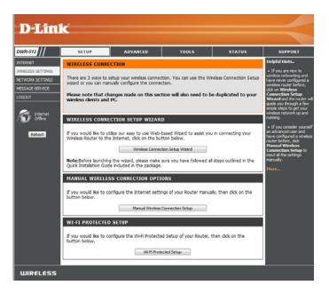
The Wi-Fi Protected Setup page allows you to create a wireless connection between your router and a device automatically by simply pushing a button or entering a PIN code.
