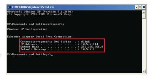
If the address is 0.0.0.0, check your adapter installation, security settings, and the settings on your router. Some firewall software programs may block a DHCP request on newly installed adapters.
