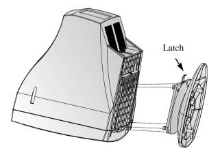
If you want to remove the tilt/swivel stand on the monitor, press the latch and pull the tilt/swivel stand toward the back of the monitor. Lift the stand to separate.
