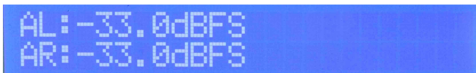
Fig. 5.6 – AES-EBU Left and Right input levels
