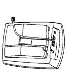
3. Insert the supplied AC adabarrel plug into the **DC 9V** ja the back of the base. Then rou cord through the strain relie and press the cord all the way into the cord groove on the b of the base.
