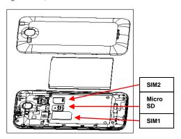
3. Finally insert the battery and replace the rear cover of the mobile phone.
