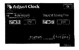
Auto Adjust ON: When you touch this switch, the time is set to the GPS clock, and this switch is highlighted in green.
