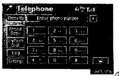
1. Touch the "Log" switch to display "Dialled Numbers" screen.
