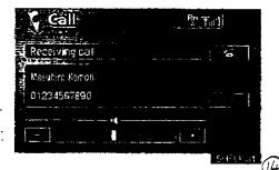
When a call is received, this screen is dis-played with a sound. Touch the "Call" to talk on the phone. You can adjust the vol-ume of received call by touching "—" or
