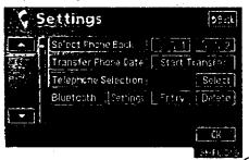
2. Touch the "Delete" switch to display "Delete Tetephone" screen. You can delete the Bluetooth phone which you registered. Select the desired phone from the list.
