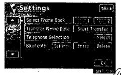
4. Touch the "Entry" switch to connect your cellular phone to the system. Input the PASS- KEY displayed on the screen.
