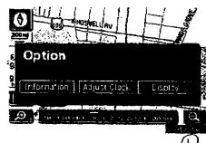
1. Push the "OPTION" button to display the "Option" screen and touch the "Information" switch.
