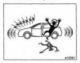
The theft deterrent system is designed to deter vehicle theft. This system flashes turn signal lights and sounds the alarm if someone attempts to damage or break into your vehicle. Furthermore, when the interior light switch is in the "DOOR" position, the interior light turns on.
