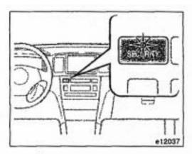
After making sure the indicator light starts flashing, you may leave the vehicle.
