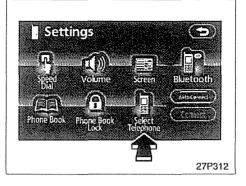
2. Touch the "Select Telephone" switch to display "Select Telephone" screen. You can select the Bluetooth phone from a maximum of 6 numbers.
