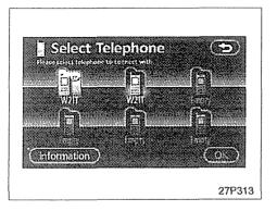
Although you can register up to 6 Bluetooth phones in the system, only one Bluetooth phone can function at a time.
