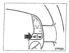
By pushing the telephone button above, you can receive a call or hang up without taking your hands off the steering wheel.
