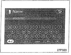
3. Use the software keyboard to input the device name.
