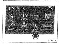
2. Touch the "Select Telephone" switch to display "Select Telephone" screen. You can select the Bluetooth phone from a maximum of 6 numbers.
