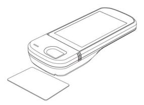
• Smart card, insert the smart card to the slot, chip should be upside.
