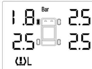
Fig 5 Low pressure alarm indication
