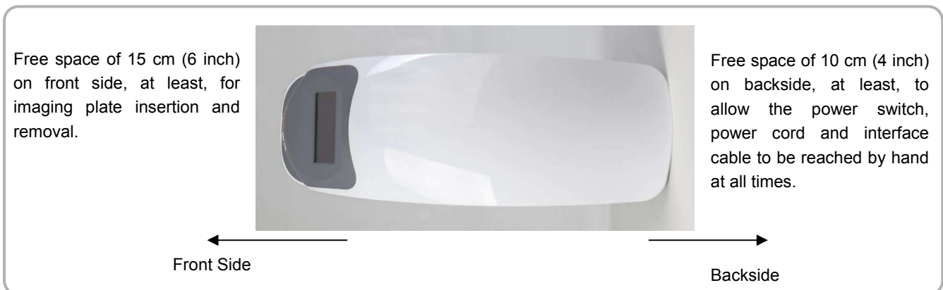
Figure 1. Space Requirements (Top View)
