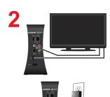
Connect the other end of the cable to the appropriate input of your TV or monitor. Confirm that both your TV and the Wireless Joey receiver are connected to a power outlet. **Note:** In most cases, connecting the HDMI cable provides plug-and-play control of the TV's display resolution and other settings. However, your TV may require selecting a different format to display from the Wireless Joey receiver during setup.
