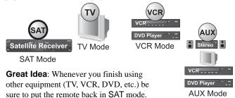
To change the mode, press the button for the equipment you want to control. The mode button lights for two seconds to show you've set the remote to that mode.
