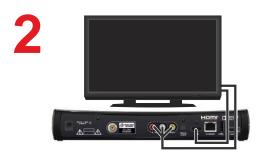
Connect the other end of the cable to the appropriate input of your TV or monitor. Confirm that both your TV and the Super Joey receiver are connected to a power outlet.
