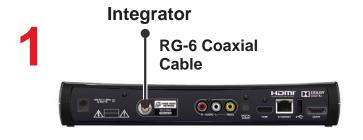
Home Video Network Port Connect one end of RG-6 coaxial cable to the **HOME VIDEO NETWORK** port on the back of the Super Joey receiver.
