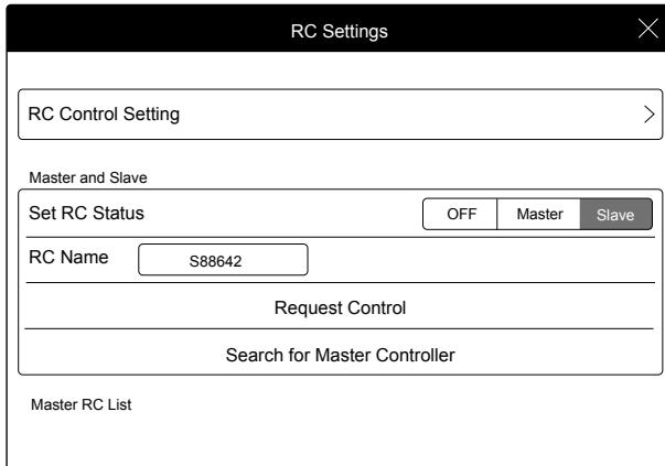
**⚠** Remote controller cannot link to the aircraft if the remote controller is set as "Slave". Meanwhile, the "Slave" remote controller cannot control the orientation of the aircraft. Reset the remote controller to "Master" in DJI GO app if you wish to link the remote controller to the aircraft.
