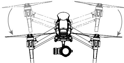
**⚠** Do not raise the landing gear when the aircraft is on the ground. Ensure the landing gear is lowered before landing.
