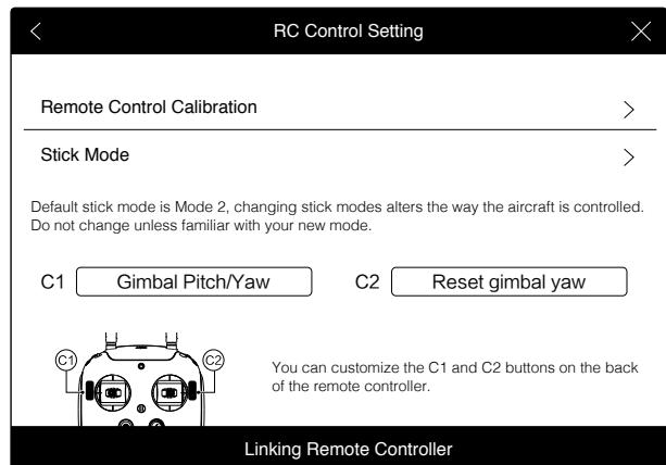
Press C1 or C2 button to switch from pitch mode to yaw mode. You may use the gimbal dial to pan the gimbal under yaw mode. Press C1 or C2 again to exit yaw mode.
