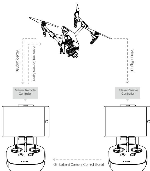
**⚠** Use the gimbal dial on the remote controller to control the pitch movement of the camera in the single remote controller mode, however, you cannot control the pan movement of the camera.
