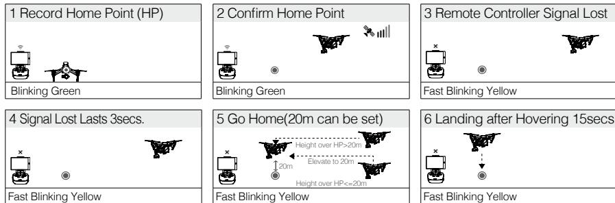
⚠ • Aircraft automatically descends and lands if RTH is triggered when the aircraft flies within a 20 meter (65 feet) radius of the Home Point.
