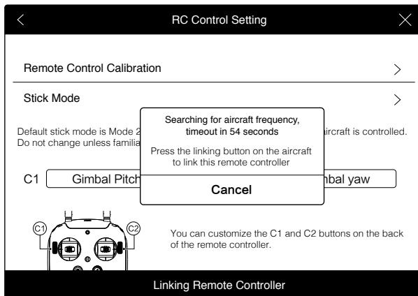
5. Locate the Linking button on the front of the aircraft, as shown in the figure shown below. Press the Linking button to start linking. The Remote Controller Status Indicator will display solid green if Link is succeed.
