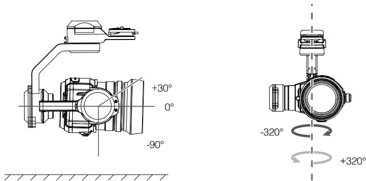
Use the gimbal dial on the remote controller to control pitch movement of the camera by default. Note that you cannot control the pan motion of the camera by default. Enable the “Master-and-Slave” mode and set the remote controller to “Slave” state if you wish to control both the pan and pitch movement of the camera.
