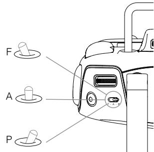
**P mode (Positioning)** : P mode works best when GPS signal is strong. There are three different states of P mode, which will be automatically selected by the Inspire 1 Pro depending on GPS signal strength and Vision Positioning sensors:
