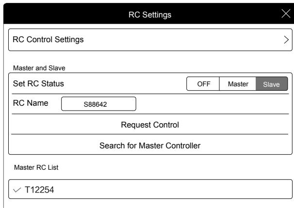
3. Select the "Master" remote controller from the "Master RC List" and input the connection password to connect to the desired "Master" remote controller.
