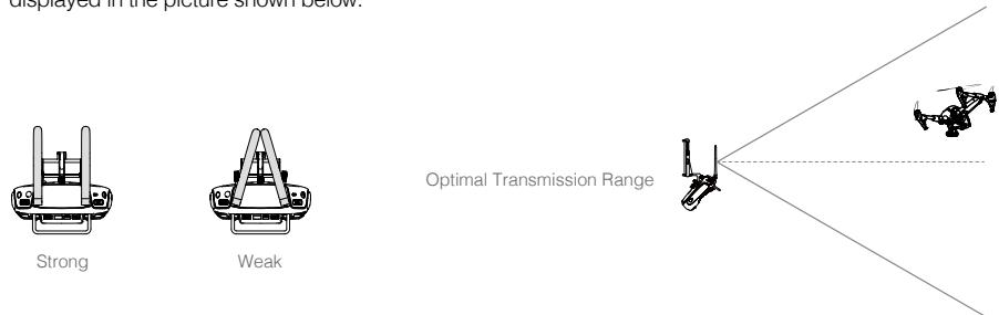
Ensure the aircraft is flying within the optimal transmission range. Adjust the distance and position between the operator and the aircraft to achieve optimal transmission performance.
