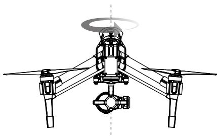
3. Hold the aircraft vertically with nose pointing downward, and rotate it 360 degrees around the center axis. Recalibrate the compass if the Aircraft Status Indicator show solid red.
