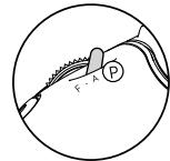
**⚠** The performance of your Inspire 1 Pro's Vision Positioning System is subject to the surface you are flying over. The ultrasonic waves may not be able to accurately measure the distance over sound absorbing materials, and the camera may not function correctly in suboptimal environments. The aircraft will switch from "P" mode to "A" mode automatically if both GPS and Vision Positioning System are not available. So operate the aircraft cautiously when in any of the following situations:
