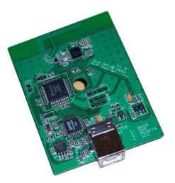
PC via the use of royalty-free Virtual COM Port (VCP) drivers. (No USB driver development is required for most applications.) The SIPP firmware in the DLP-RF1 resides at the application layer and is based on Freescale's SMAC. The SIPP firmware provides basic access to DLP-RF1 functionality: packet receive and transmit, transceiver settings, EEPROM access, etc.
