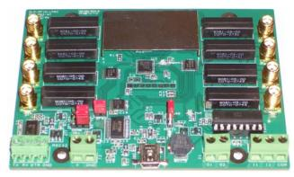
the DLP-RFID-LP8C's electronics reside on a single compact PCB, and all operational power is taken from the host Windows/Windows CE/Linux PC via the USB interface. Up to 8 external antennas can be connected via standard SMA connectors.
