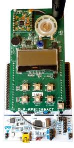
This section describes how to operate the DLP-RFS1280ACT demonstration hardware. This hardware includes a DLP-RFS1280 transceiver module, allows the operator to easily verify normal operation of the transceiver and assists in learning the operational firmware.
