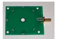
This antenna is well suited for reading the near-field loop incorporated into many Gen-2 tags. This antenna requires a coax cable with a reverse-polarity SMA connector at one end for connection to the DLP-RFID-UHF1B reader. A 3-foot coax cable is provided with each DLP-RFID-UHF1B reader purchased from DLP Design.
