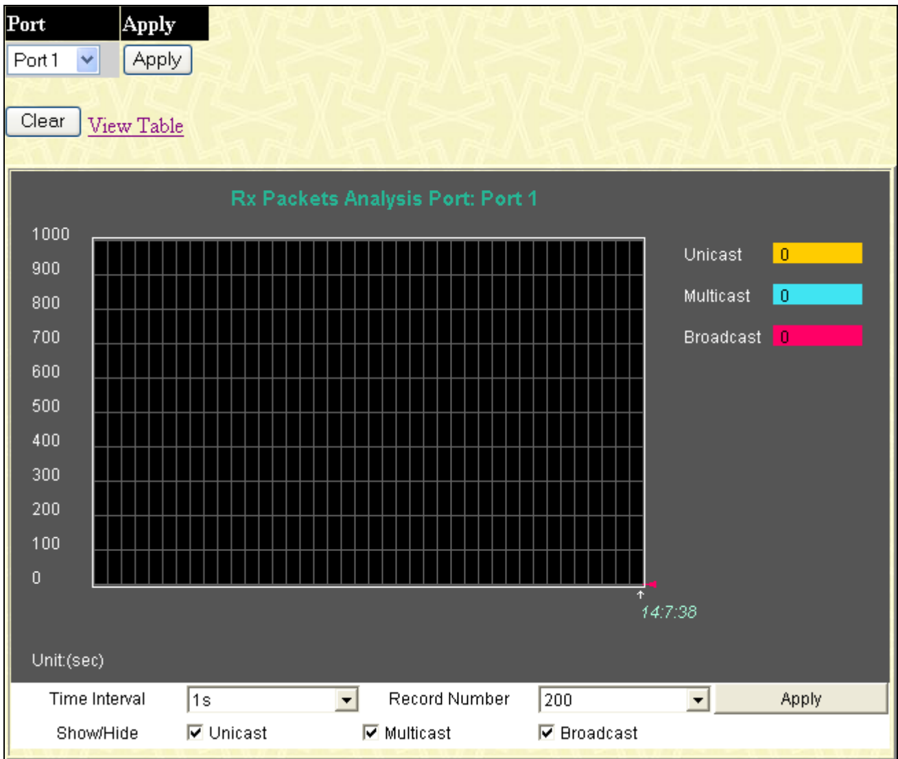
Figure 11- 5. Rx Packets Analysis window (line graph for Unicast, Multicast, and Broadcast Packets)
