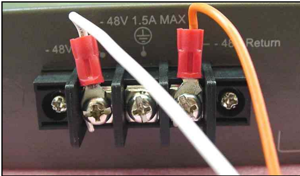
Figure 2- 7. Power connections attached to contacts on assembly
