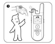
4、 键盘锁: 往下拨动解锁 Security Keypad Lock: Toggle it down to unlock.
