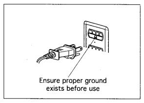
For a permanently connected appliance: This appliance must be connected to a grounded, metallic, permanent wiring system, or an equipment grounding conductor should be run with the circuit conductors and connected to the equipment grounding terminal or lead on the appliance.
