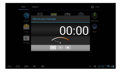
In the recording interface, touch " to start recording, after the recording is finished, touch " to save automatically. The recorded files will be saved in the "Recordings" file folder under root directory in "recordingxxxxx.mp3" file format. All the recording files can be played in the music play mode.
