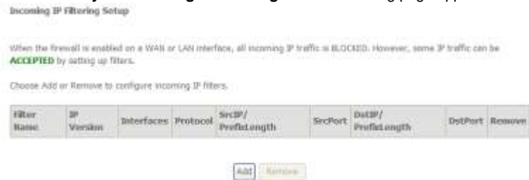
Figure 82 Incoming IP filtering setup
