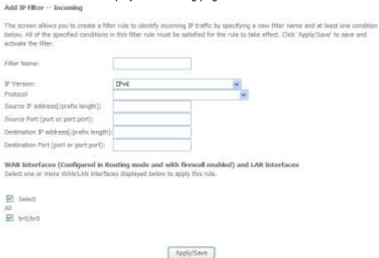
Figure 83 Adding an IP incoming filtering rule
