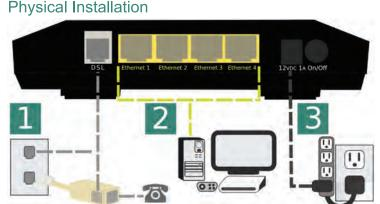
1 Connect DSL Port to Phone Jack If a dual port filter is provided, and you would like to use a phone with same wall jack used for your gateway, connect the dual line filter to the wall jack. Next, connect your Gateway's "DSL Port" to the "DSL Port" of the filter; and your phone to the "Phone" port of the filter.
