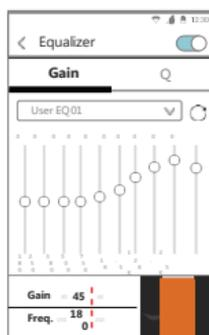
5. Press [Q] tab on top to view the PEQ setting screen.
