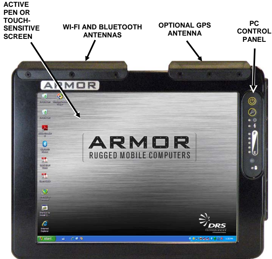
Figure 2. ARMOR X10 Key Features – Front View
