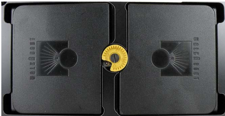
Figure 19. Battery Latch in Locked Position
