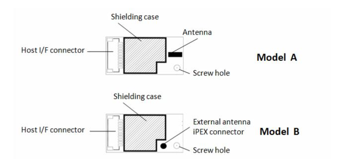
**Model A:** the chip antenna is embedded on board.
