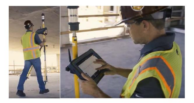
The distance is exceed 20cm between DT301A mobile tablet and the body of operator that ensure the precision and accuracy of measurement.
