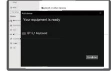
1. Turn on the device, the blue light shining one time, then press Button of Connect with 3 seconds, the blue light Twinkle, so that means the keyboard in the matching status. after maching succeed, the twinkle blue light off, fold close the keyboard, the Power off.
