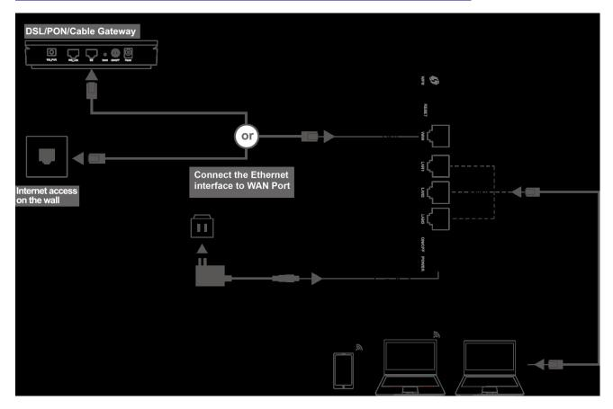
The DZS Router can be connected according to the diagram above.
