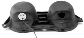
10. Install the lens and/or re-assemble the tail light housing, insuring all gaskets are intact and in place. Install the tail light housing back into the vehicle. You are now ready to wire the LED assembly into the vehicle tail light harness.
