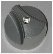
1. Carefully remove the rubber plug from the center of the headlight switch cover as it will be reused in the new switch cover. A needle nose pliers works well for this.
