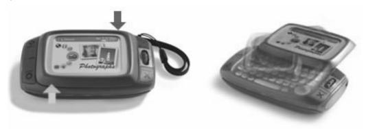
2 To close the display lid, reverse the motion to pivot the lid counter-clockwise and lock it into the closed position.
