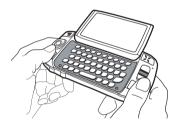
Alternatively, use your right index finger to push down gently on the upperright corner of the display. The screen will spring into the open position.
