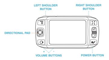
**DIRECTIONAL PAD (D-Pad)** Press up/down/left/right to scroll or move within text fields, and navigate in games. The D-Pad "rocks" into four different directions or positions.
