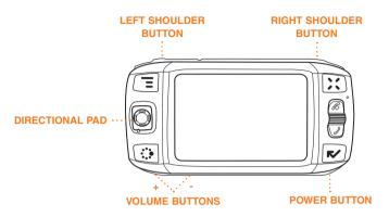
**DIRECTIONAL PAD (D-Pad)** Press up/down/left/right to scroll or move within text fields, and navigate in games. The D-Pad "rocks" into four different directions.
