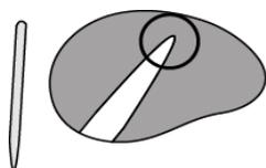
Step 4: To begin activation, first press the CONNECT button on the receiver, and then (using the pointed object) press the CONNECT button located on the bottom of the mouse within 3 seconds of each other.
