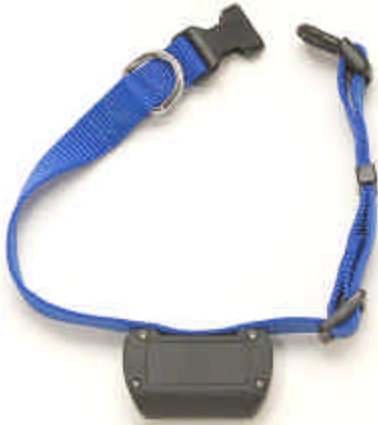
The Large Animal Telemetry Repeater's design allows it to be attached to an animal's collar, secured on a harness, or in a vest pocket.
