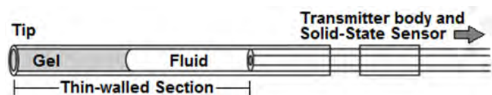
Detailed diagram of catheter components with the tip cover removed
