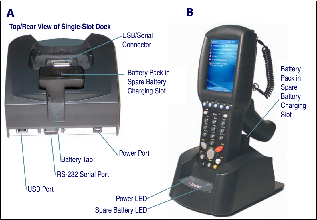
Figure 8. Charging the Battery Pack in a Single-Slot Dock
