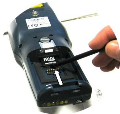
To remove the Mini SD card, just push it toward the inside, aided by the stylus, until it clicks; a spring system will return it out.
