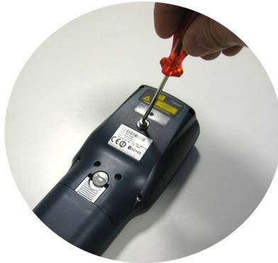
2. Screw the belt clip pivot on the terminal by using the fixing screw.
