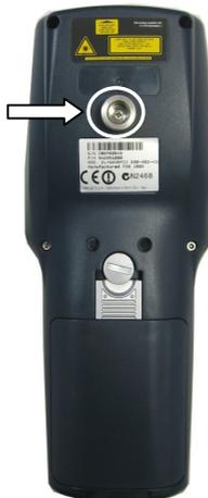
3. Insert the terminal in the belt clip by sliding the belt clip pivot into the belt clip until it clicks into place.
