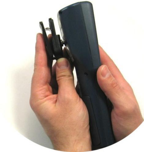
4. To release the terminal, press the belt clip unlock button.
