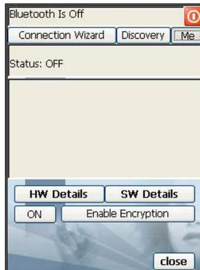
By tapping on the “HW Details” and “SW Details” buttons, information about the mobile computer Bluetooth® hardware and software will be displayed, while the “Enable Encryption” button starts encryption of the Bluetooth® communication data. If tapping on the “Close” button the Bluetooth® Manager Device window will be closed.
