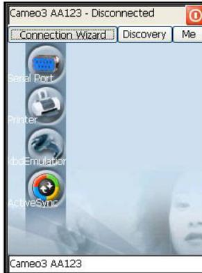
3. Tap on the “Me” button to enter the related window; then, tap on the “ON” button to activate the Bluetooth® module. The module activation may be also performed by using the WIRELESS COMMUNICATION applet as described in par. 3.7.4.
