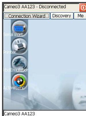
The “Serial Port” button starts communication through the Bluetooth® serial port COM 5.
