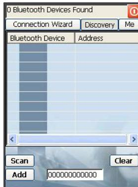
Once the Discovery procedure has been completed, select the desired Bluetooth® device from the list. It is also possible to digit (12 hexadecimal digits) the Bluetooth® address of the desired device by tapping on the “Add” button. The “Clear” button deletes all discovered devices from the list.
