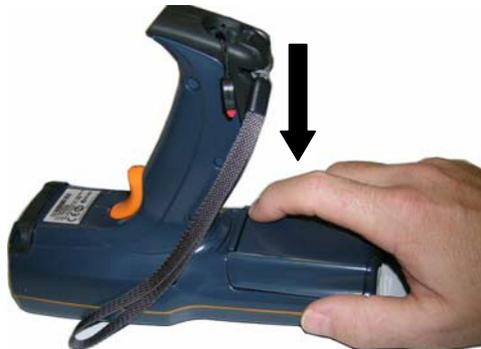
4. Press it until the battery latch is automatically closed.
