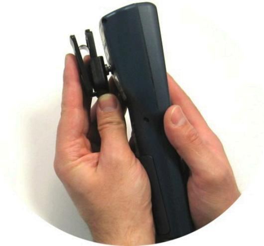
4. To release the terminal, press the belt clip unlock button.
