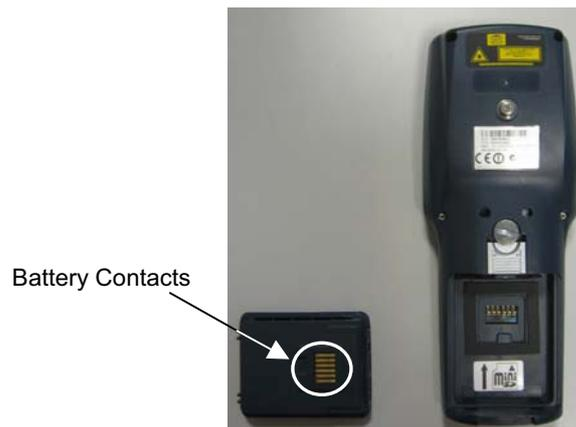
4. To correctly insert the new battery pack, first insert the bottom and then the upper part of the battery pack into the slot as indicated in the following figure:
