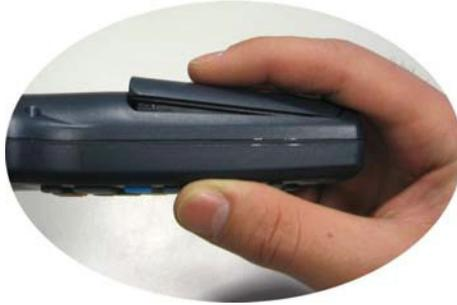
5. Press it until the battery latch is automatically closed.
