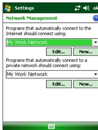
then ensure that the USB/Ethernet Adapter card connects to Work -> go to Start -> Settings -> Connections -> Network Cards:
