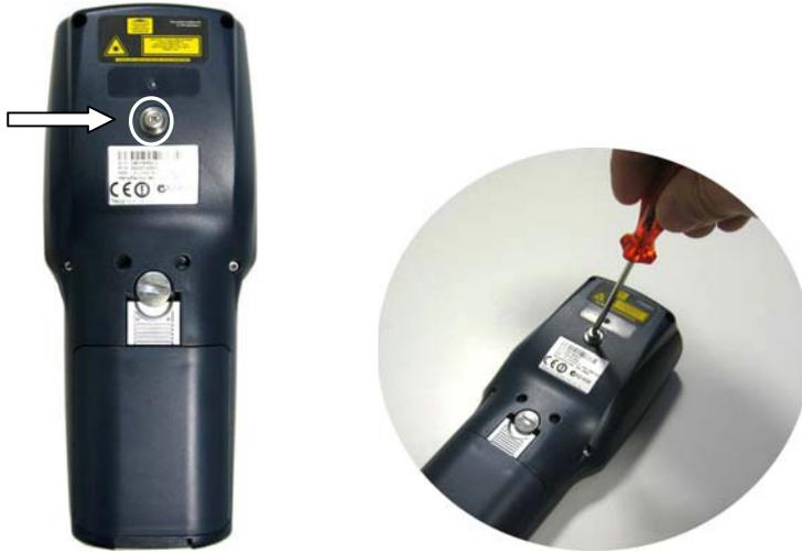
2. Screw the belt clip pivot on the terminal by using the fixing screw.
