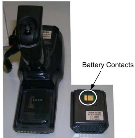
3. To correctly insert the new battery pack, first insert the bottom and then the upper part of the battery pack into the slot as indicated in the following figure:
