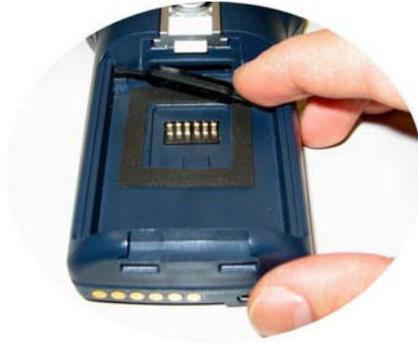
3. Insert the card with the written part upward (as shown in the figure) and push it in, aided by the stylus, until it clicks into place.
