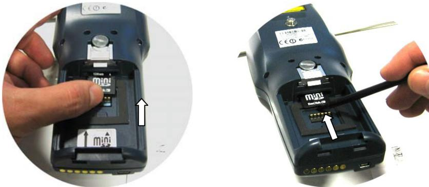
To remove the Mini SD card, just push it toward the inside, aided by the stylus, until it clicks; a spring system will return it out.
