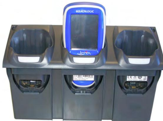
JOYA Cradle Dispenser has three JOYA™ X1 slots, each equipped with its own control unit, an electromechanical system for blocking/releasing the terminal, notification light, battery power and recharging circuits. Its special structure makes it possible to design any type of dispenser (wall-mounted or island) easily, allowing twice the number of terminals to be installed per vertical square meter with respect to the competing systems.
