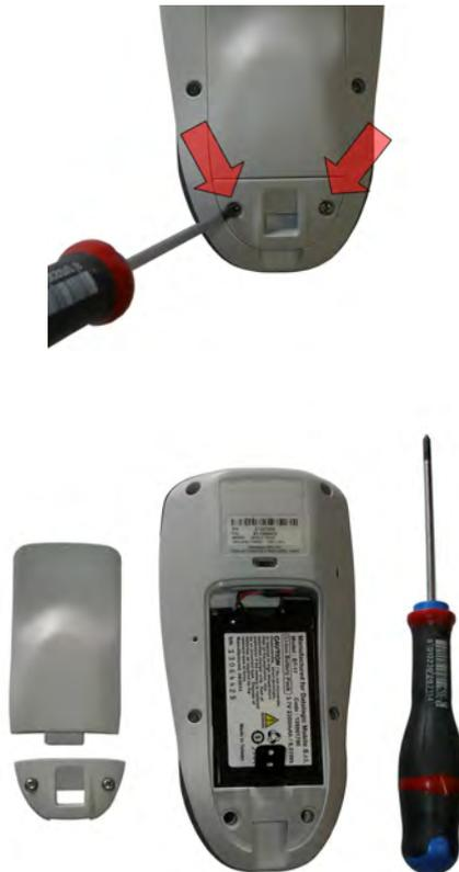
2. Remove the cover and then the battery pack, using the proper plastic strips. Pay attention when disconnecting the connector.
