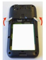
2. Insert the battery pack into the slot, bottom first, and press it into place:
