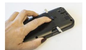
3. Rotate the latches to the lock position to lock the cover:
